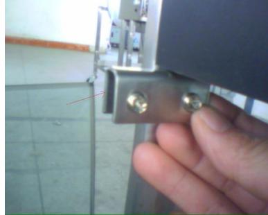
3. Place the left side top door hinge assembly into the upper frame left hole slot and proceed to slide and insert the complete glass door into the top door hinge. Please note the arrow direction in the figure above. Once in place slide supplied gaskets in between door hinge assembly and glass door making sure white gasket is in behind door hinge with screws and tighten loosely.
